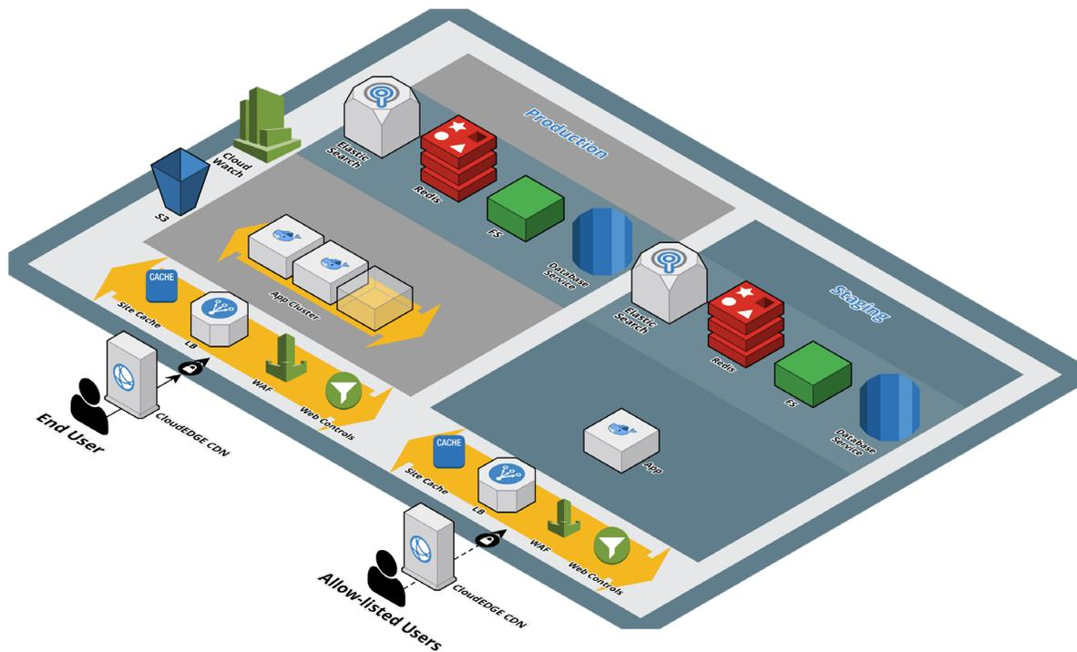
In Webscale’s decentralized architecture, the stateless application tier scales to a pre-set maximum depending on traffic demands. This configuration is based on a deployment within the public cloud to reduce overall costs and to take advantage of rapid scaling capabilities, if needed.
